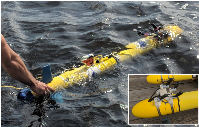
Fig. 6: Photo of our commercial Bluefin SandShark miniature AUV outfitted with a custom pyramidal iUSBL hydrophone array mounted above the nose (inset).
