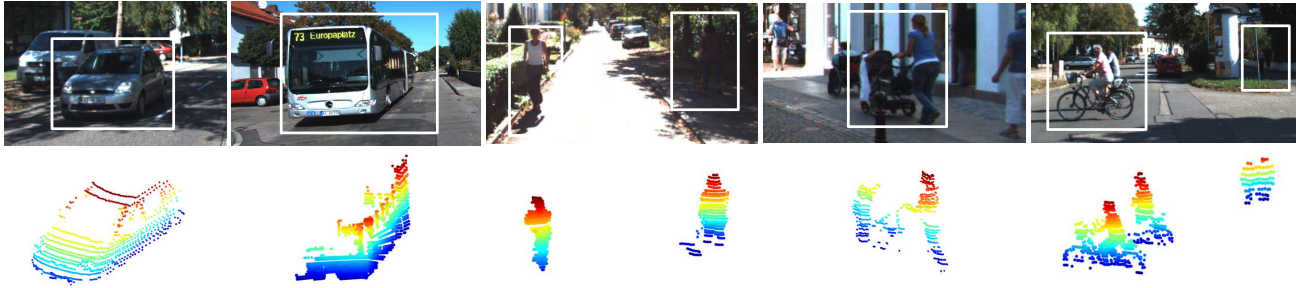
Fig. 10: Examples of self-parsed urban dynamic objects, which are automatically extracted from various sequences of the KITTI dataset. From left to right, the objects are a car, a bus, a pedestrian, a pedestrian with a dog, a pedestrian pushing a stroller, bikes, and a pair of pedestrians. As mentioned in Fig. 5, our method does not assume any model's shape, size, or density and does not require point cloud processing (e.g., ground removal, normal estimation, or region growing).
