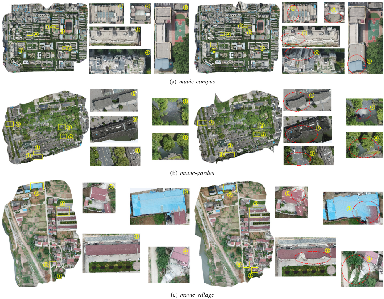
Fig. 6. Orthomosaic results comparison between DenseFusion (left) and TerrainFusion (right). TerrainFusion generates acceptable result in low elevation offset areas but outputs twisted details for buildings. Benefit from the dense reconstruction, details of DenseFusion looks much better.
