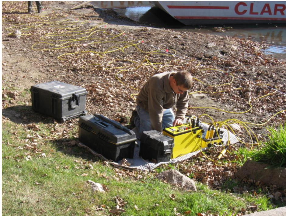
Figure 7. IGWS conducting geophysical survey at East Okoboji Lake shoreline. Yellow cables are attached to numerous stainless steel stakes. Electric current is directed through the cables and into the ground via metal stakes. This is a highly effective method to characterize the lateral variation and extent of sediment packages with highly varying resistivity ie. coarse-grained vs. fine-grained deposits.
