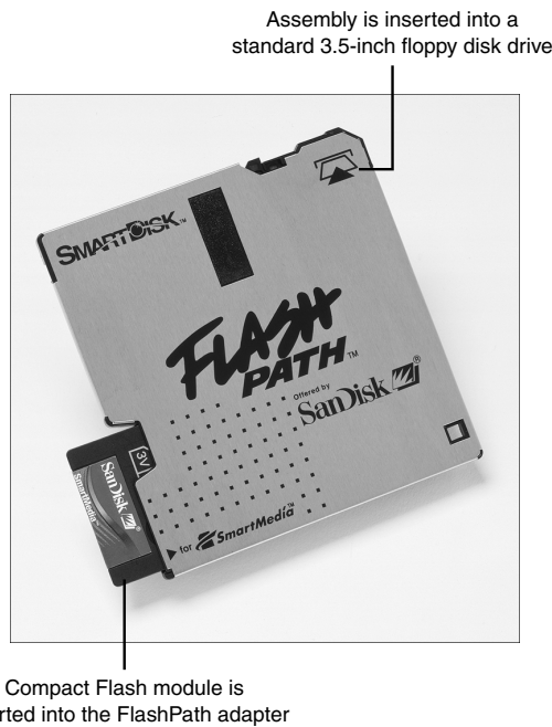
Figure 12.6 A CompactFlash module is inserted into the FlashPath adapter; the assembly is then inserted into a standard 3 1/2" floppy drive. Photo courtesy of SanDisk.
