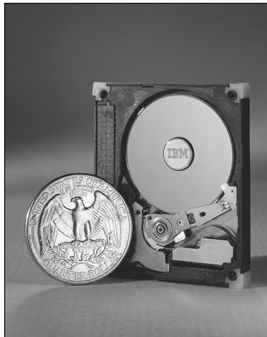
Figure 12.7 A U.S. quarter is just slightly smaller than the Hitachi (originally IBM) Microdrive. Courtesy of International Business Machines Corporation. Unauthorized use not permitted.
