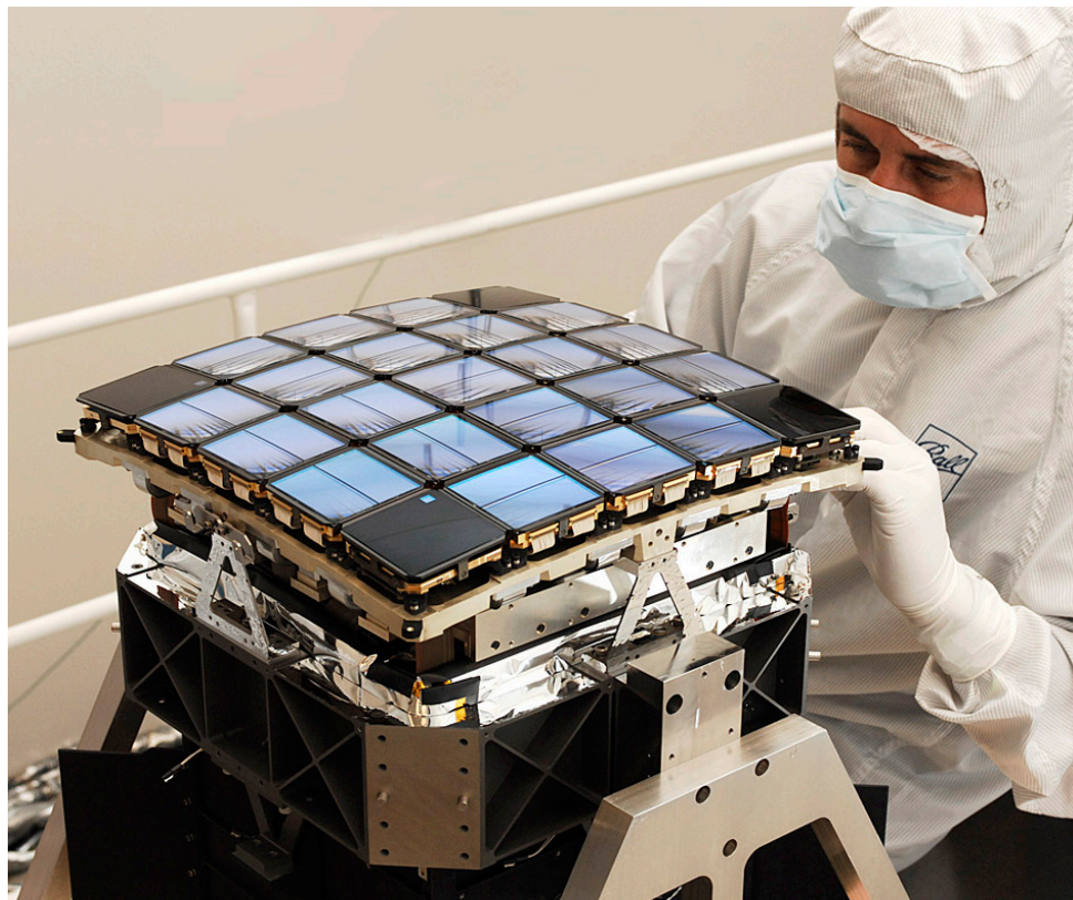
Completed flight focal plane array with the 42 science CCDs and four fine guidance CCDs in the corners.
