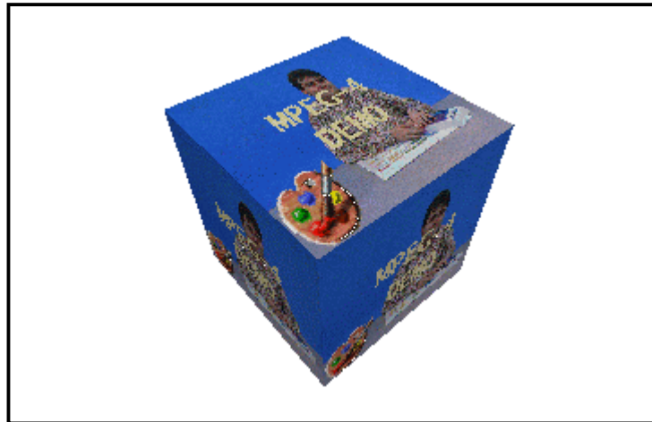
Figure 16 - A CompositeTexture2D example. The 2D scene is projected onto the 3D cube.
