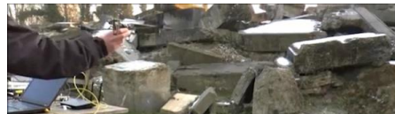
RMS error: 5 mm, height: 1.5 m – Down-looking camera
