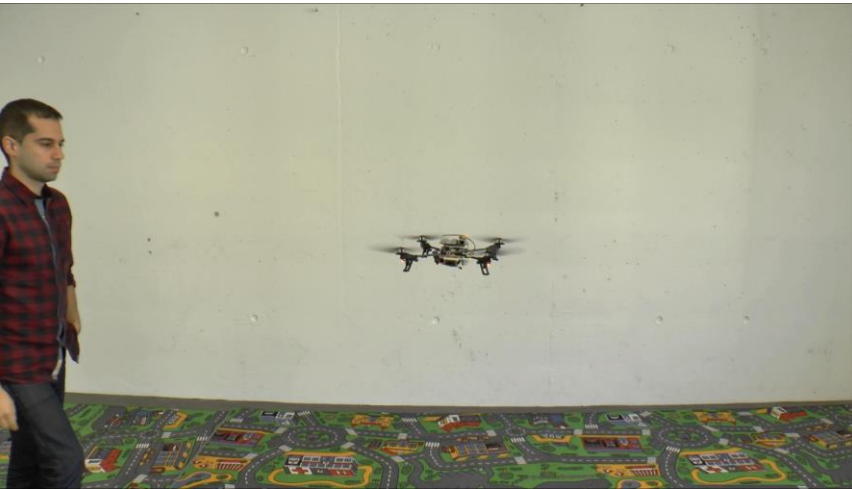
RMS error: 5 mm, height: 1.5 m – Down-looking camera
