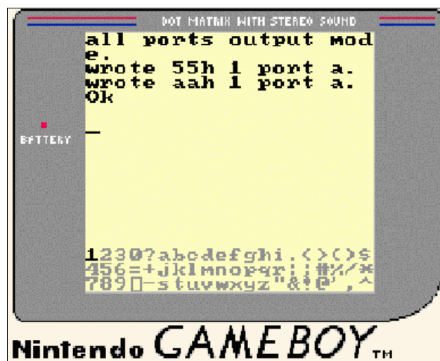
Figure 18: GBBasic accessing the 82C55A
