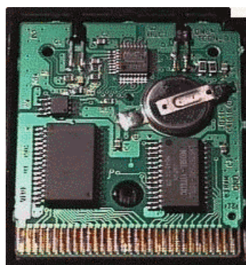
Figure 1: Inside a cartridge (Type 10h)
