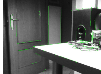
Fig. 1. In low-textured environments, point-based algorithms usually fail due to difficulties in founding a large number of features, in contrast, line segments are usually abundant.
