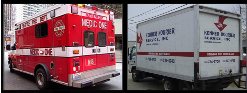
Figure 26 Current ADAS often struggle to differentiate between Ambulances and similar looking trucks
