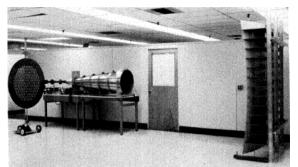
Fig. 4. Microwave power transmission laboratory experiment in 1975 by W.Brown.
