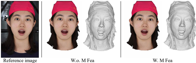
Figure 11. Illustration of the location of geometric features in the rendering module of the neural multi-view framework. The middle is the result of the usual feature extraction location, and the right is the result by changing the extraction location to the connected layer.
