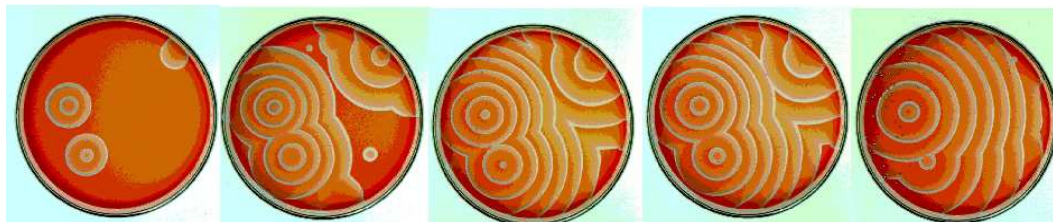
Figure 2.11: Wavetrains in a BZ system in excitable state. The diameter of the dish is 9 cm. The frames were taken at 1 min, 3 min 30 s, 7 min 15 s, 7 min 35 s and 16 min 20 s after the mixing of the solution [33].
