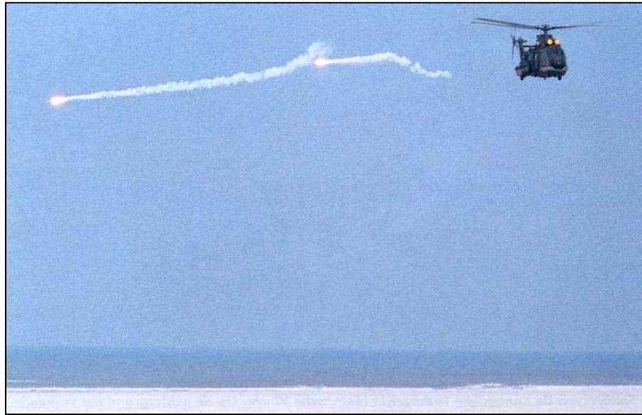
A Dutch Cougar helicopter ejects two flares above the North Sea. This type of flare is used to deviate heat-seeking missiles (source: Onze Luchtmacht , vol. 51, N°3, June-July 1999, p.40)
