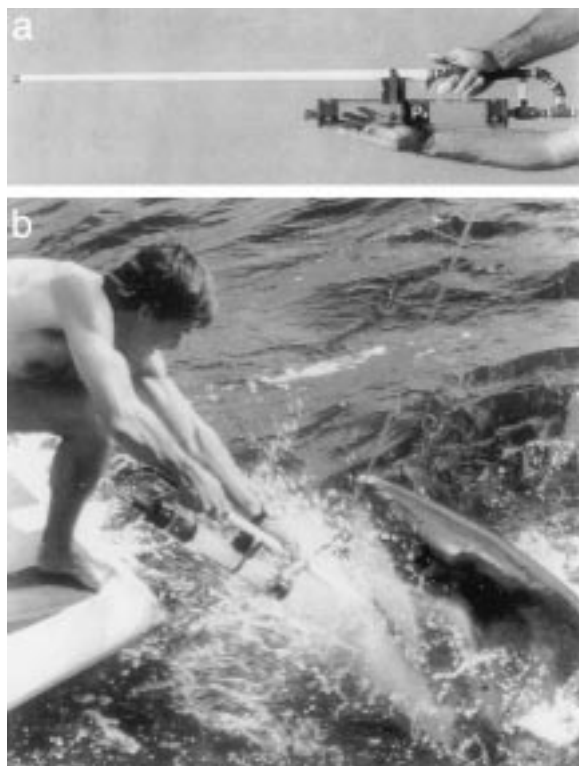
Figure 7. 'Chemical enhanced' shark billy club developed by D.R. Nelson that can deliver a rapid squirt of sodium dodecyl sulfate (SDS) to repel sharks. a – The device contains 250 ml of the SDS test solution to the right of the piston (P) and 60 psi of compressed air to the left of the piston. The device (122 cm in length) is discharged by a thumb operated valve that allows the compressed air to drive the cylinder piston to the right, thereby pushing surfactant solution out of the barrel in approximately 1 s (photograph courtesy of W.R. Strong). b – Shark researcher W.R. Strong tests the 'chemical enhanced' shark billy club on a bait-attracted white shark from the stern platform of the R/V Alcyone (photograph courtesy of the Cousteau Society).
