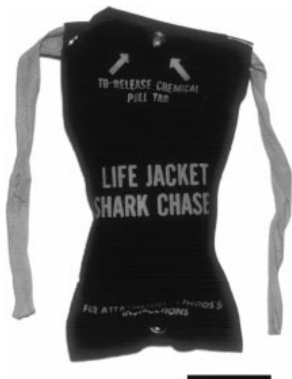
Figure 1. Shark Chaser, the original U.S. Navy chemical 'shark repellent', was primarily a package of copper acetate and nigrosine dye issued to all naval personnel but later proven to be ineffective against repelling sharks. Scale bar = 5 cm.
