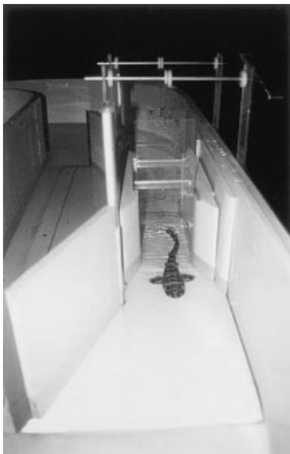
Figure 4. Test chamber used to test surfactants as chemical shark repellents on swell sharks, Cephaloscyllium ventriosum .
