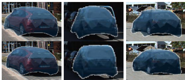
Fig. 8: Top: category-level model before shape optimization. Bottom: instance-level model after shape optimization.
