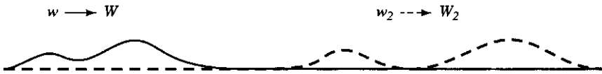
Figure 2.1 Russell's picture of the decay of one solitary wave into two waves moving with different velocities in the same direction
