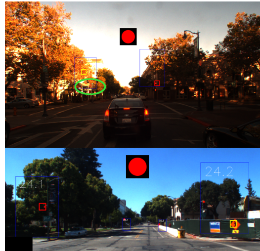
Fig. 13. Considering multiple lights with separate search windows (here, shown in blue) improves robustness. In the top frame, the window on the left reports a yellow light with 38% probability and the window on the right reports a red light with 53% probability. The final state decision of the intersection, taking into account probabilities for red, yellow and green states from both windows, yields (correctly) a red state with probability 53%. A green ellipse surrounds the actual red light that we missed, illustrating how difficult the problem is. In the bottom frame, probabilities are 80% and 48% for the left and right lights and 87% for the intersection, whose state is correctly detected as red.
