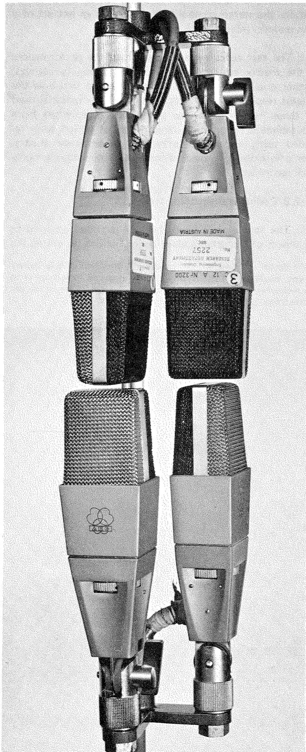
Fig. 1 - Coincident cardioid microphone array
