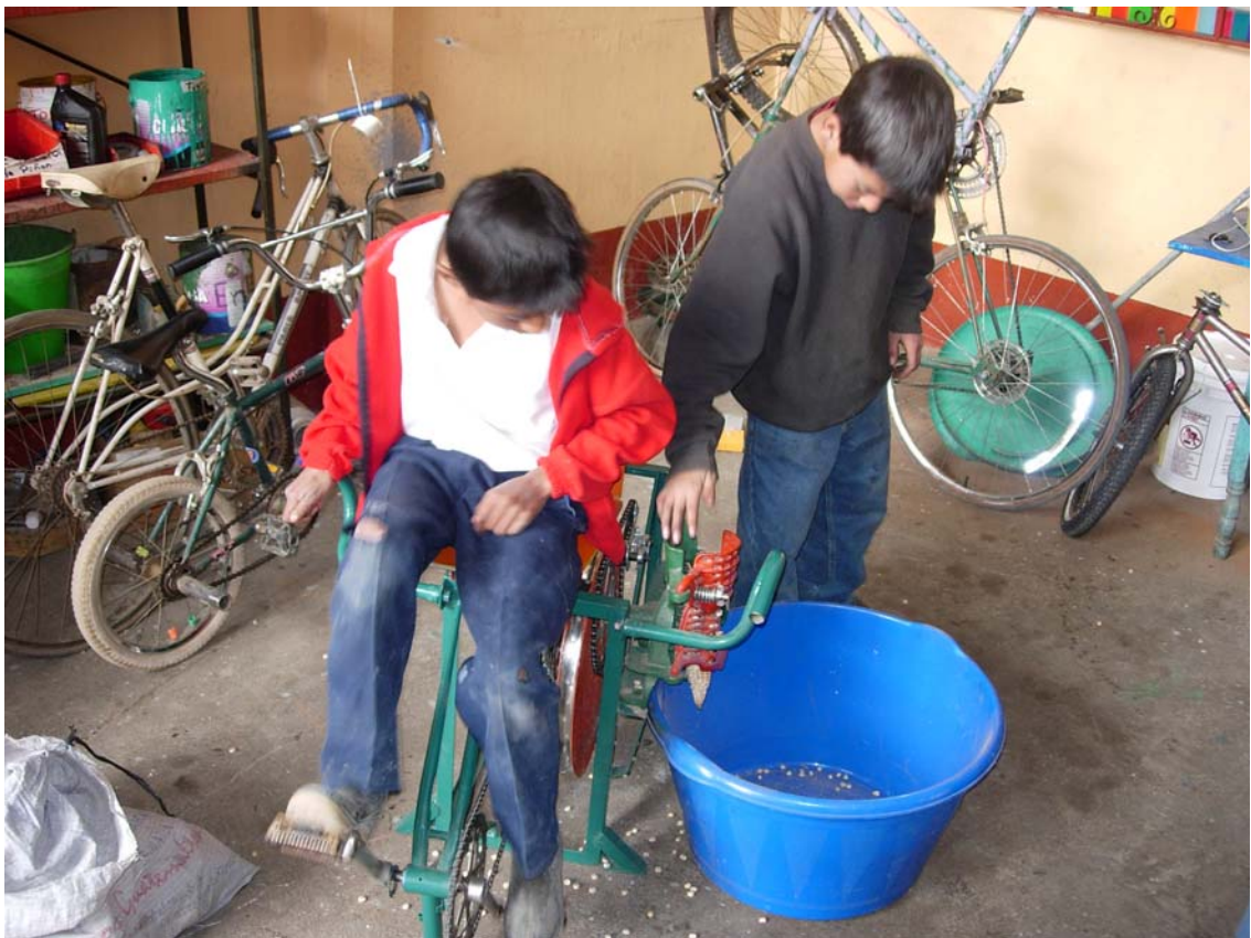
Figure 17-Extracting Corn with a Machine Designed by Maya Pedal
