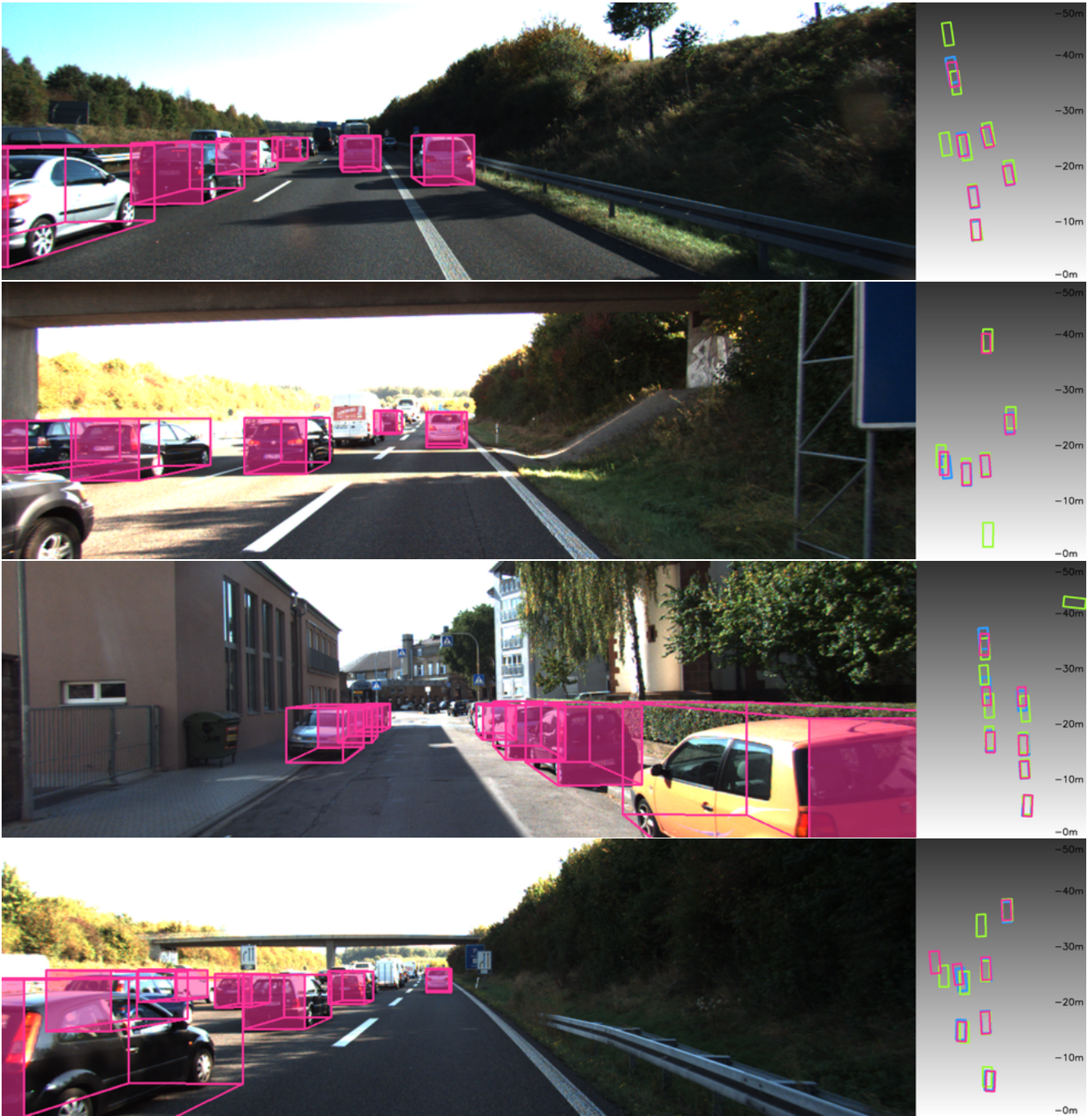
Figure 6: Qualitative Results (Best viewed in color). We depict the predictions of GrooMeD-NMS in image view on the left and the predictions of GrooMeD-NMS, Kinematic (Image) [12], and Ground Truth in BEV on the right. In general, GrooMeD-NMS predictions are more closer to the ground truth than Kinematic (Image) [12].
