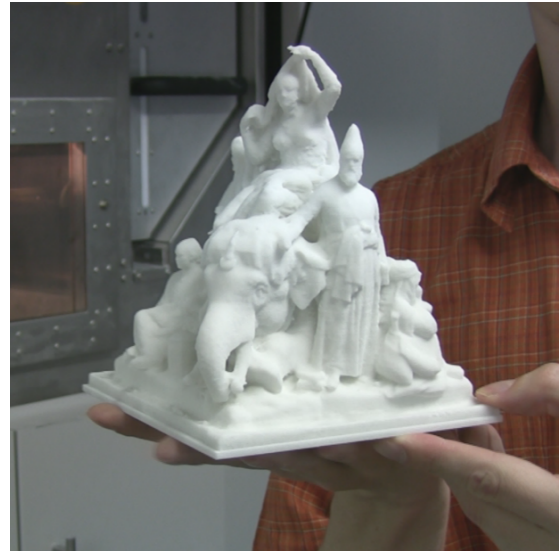
Fig. 1. A replica of the Asia statue produced with rapid prototyping from a 3D model created by our pipeline from 238 input images.
