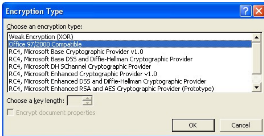
Illustration 8 Encryption method can be chosen in Encryption Type dialog called by the Advanced button of the security dialog
