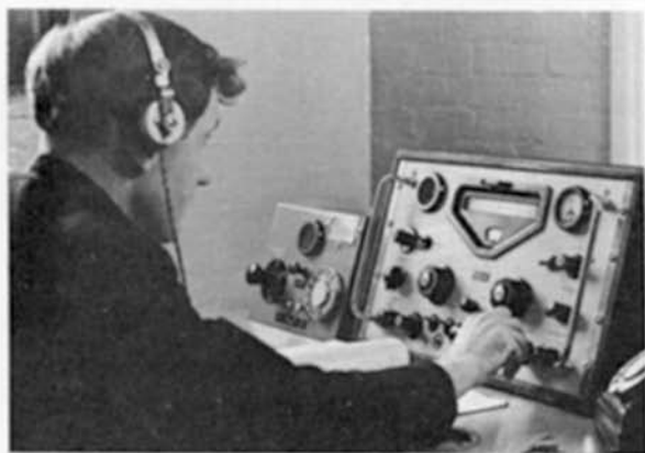
One of the five monitoring cubicles: To the left of the receiver are the programme selector dial and small loudspeaker, and the aerial switch.
