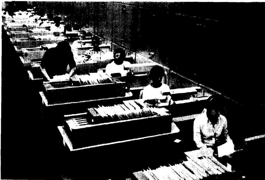
On this multiple position-letter sorting machine, clerks can mechanically sort about 1,800 pieces per work-hour. (U.S. Postal Service photo)
