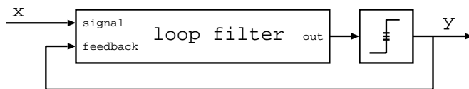
Figure 2.3: Generic model of the Sigma-Delta noise-shaping loop, consisting of 2-input loop filter and quantizer.
