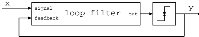
Figure 5.1: Generic model of the Sigma-Delta noise-shaping loop, consisting of 2-input loop filter and quantizer.
