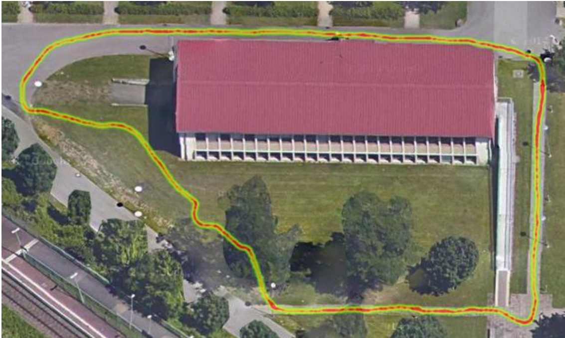
Figure 3.18: Map showing one of the trajectories that the robot followed during the classification experiments using a mobile phone microphone mounted on the robot. The variation in the robots speed along the path is shown as a heatmap on the trajectory. Thicker red lines indicate slower speed.
