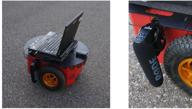
Figure 3.2: The Pioneer P3-DX platform equipped with a shotgun microphone with an integrated shock mount that we use in our experiments. The microphone is mounted close to the wheel with the supercardioid pointing towards the tire-terrain interface.
