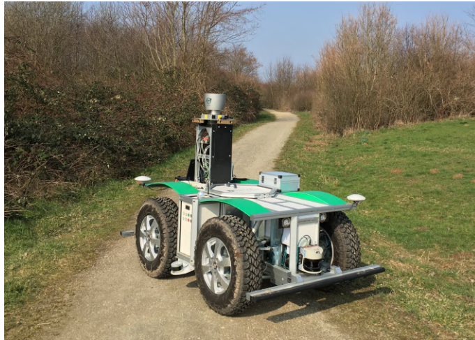
Figure 4.9: The Viona robot platform that we used for data collection equipped with a Bumblebee2 stereo vision camera and a self-made NIR camera. Both the cameras were time synchronized and the images were captured at 20 Hz.
