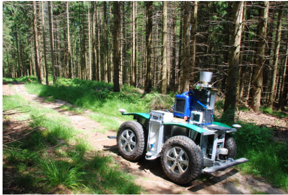
Figure 5.17: Our Viona robot autonomously navigating in a forested environment near Freiburg using our multimodal semantic segmentation network for perception. The robot was equipped with four Bumblebee2 stereo cameras mounted in perpendicular directions and an NVIDIA Jetson TX1 for the computation.
