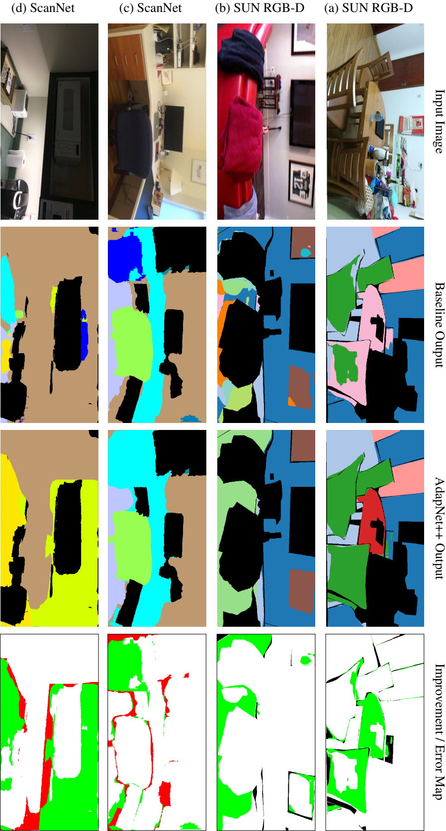
Figure 4.20: Qualitative segmentation results of our AdapNet++ architecture in comparison to the best performing state-of-the-art model (DeepLab v3) on SUN RGB-D and ScanNet datasets. In addition to the segmentation output, we also show the improvement / error map which indicates the misclassified pixels in red and the pixels that are misclassified by the best performing state-of-the-art model but correctly predicted by AdapNet++ in green. The color legend for the segmentation labels correspond to those shown in the benchmarking tables in Section 4.4.1.
