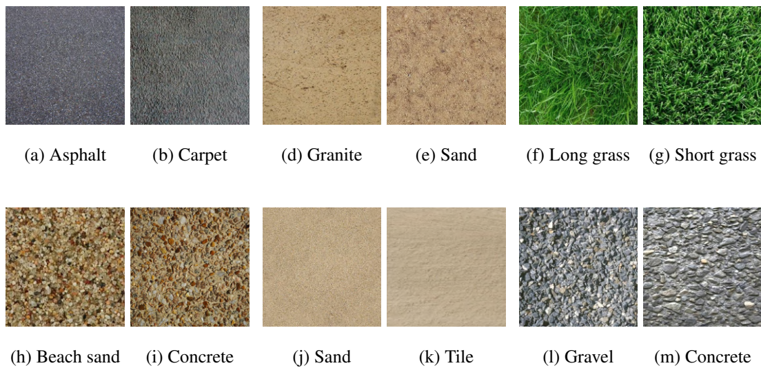
Figure 3.1: Ambiguous appearance of terrains that make traversability analysis using optical sensors extremely challenging. Visually similar terrains having different traversability properties are shown in pairs.
