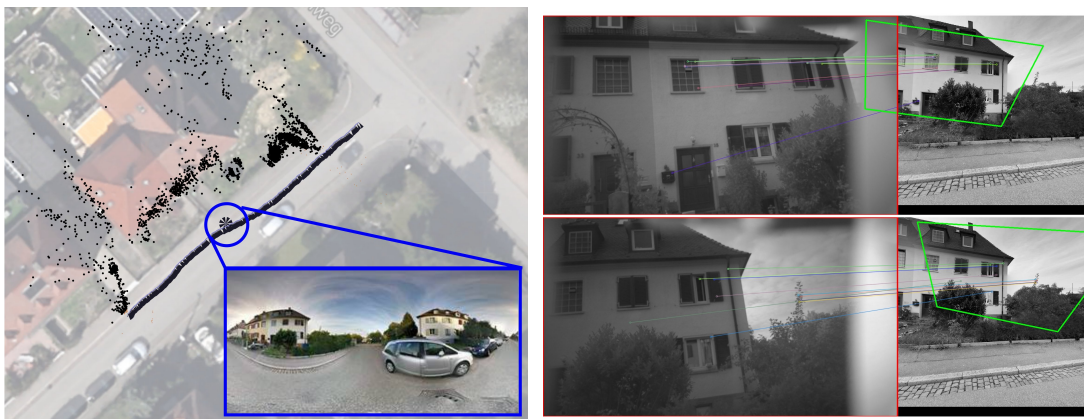
Figure 7.10: Optimized 3D points with the estimated panorama position overlaid on Google maps (top). An example of matching between panorama views and Google Tango images. As both cameras are pointing in different directions, the features used internally for visual inertial odometry are different from the features used for localizing Street View panoramas.
