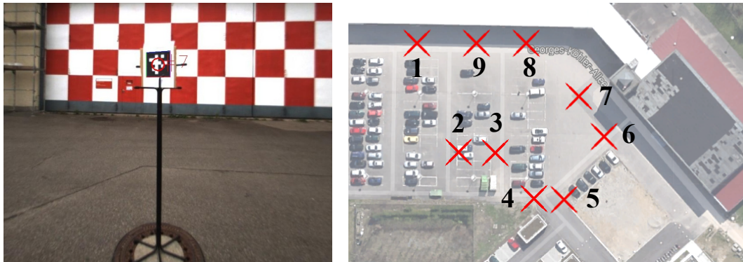
Figure 7.5: The left figure shows an example of an AprilTag placed above a manhole from where a panoramic image was acquired. The right figure illustrates an aerial view of the parking lot for the parking lot experiment. Red crosses highlighting the positions of the panoramas. The numbers represent the AprilTag ID.
