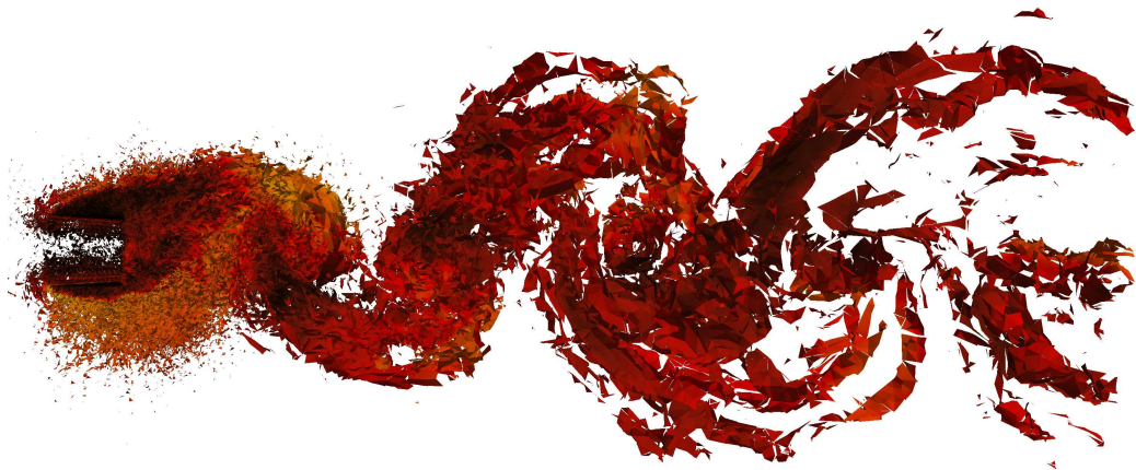
Figure 2.21: Isosurface of the q -criterion colored by velocity magnitude showing the wake behind the square cylinder
