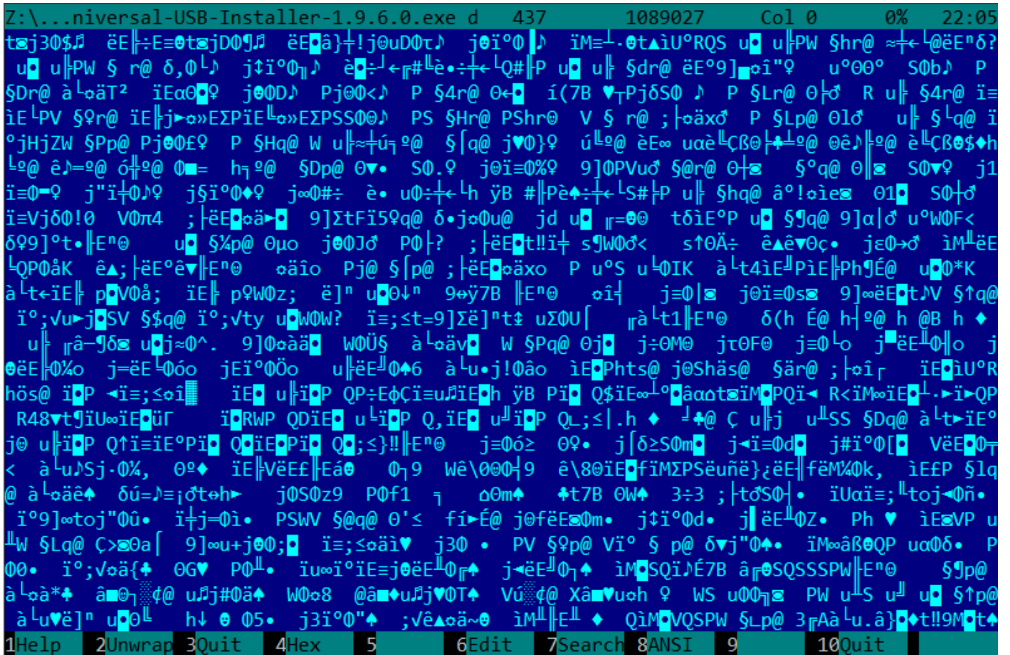
Figure 5.13: FAR: Executable 32-bit x86 code
